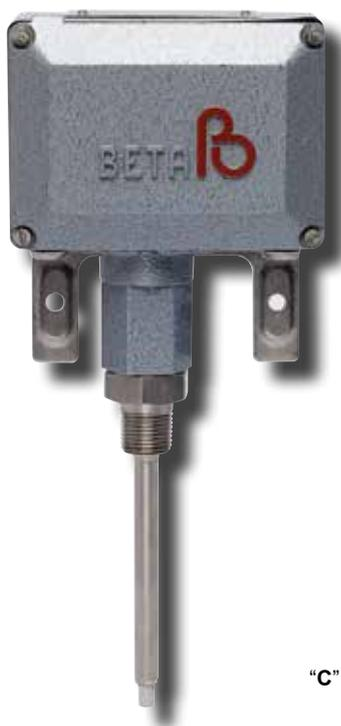
The BETA Temperature Switch is a pressure switch enclosure incorporating a sealed 2-phase (vapor/liquid) temperature sensor. When the temperature of the process increases, the vapor pressure of the liquid also increases.
